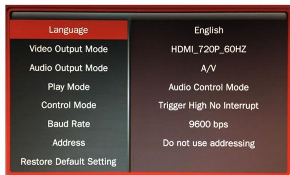
Setup menu for PIR trigger of audio playback.
